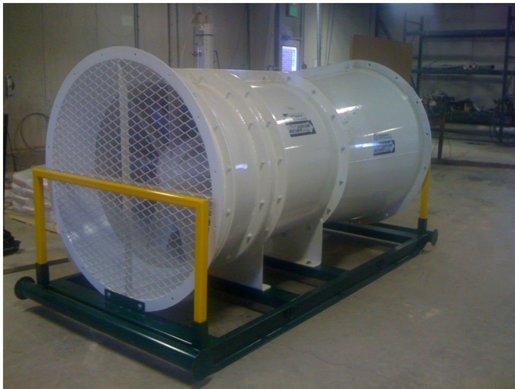
Figure 7.6. Completed skid with the mounted booster fan
