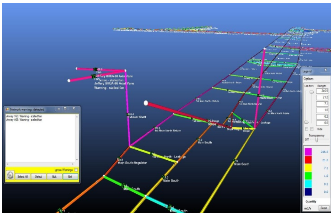
Figure 5.4. Ventsim Visual schematic view of exhaust shaft #2
